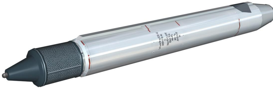
Figure 40. The S-25 Unguided Rocket in its Launch Tube
