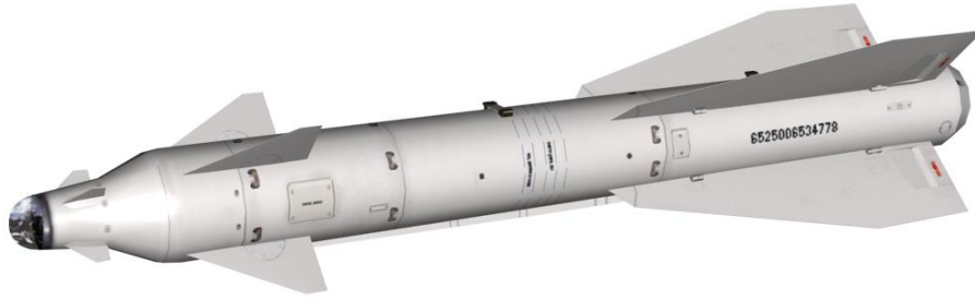
Figure 26. The Kh-29L (AS-14 "Kedge") Tactical Missile
