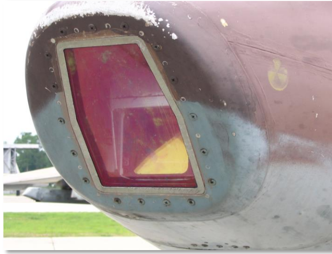
Figure 22. Nose of Su-25 with laser range finder "Klen"
