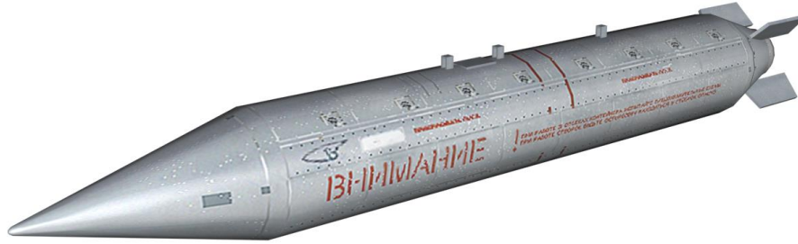
Figure 35. The KMGU-2 Sub-munitions Dispenser
